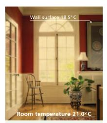
After internal insulation: Warm walls make for a comfortable room climate even at lower temperatures
